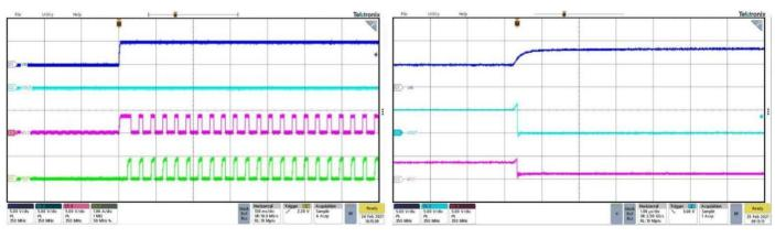
power up with output short circuit
