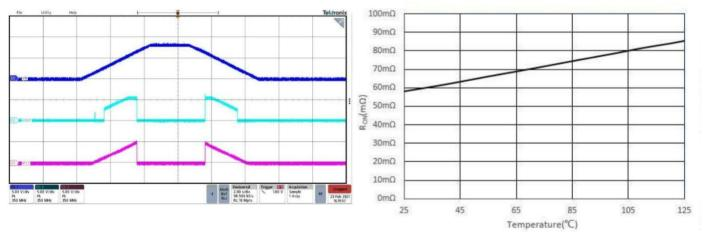
**Output Clamp as Input Ramps up**
