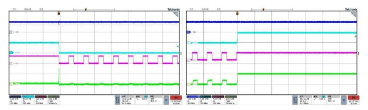
output short circuit with 2.5  $\Omega$  load
